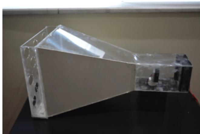
The dust sensor was placed at the end of the box, while a fan was added to the other end to increase the airflow rate through the tunnel. To house the dust sensor circuitry, I designed and 3D-printed a black enclosure. This box not only protected the circuitry but also served as a leveling base for the testing tunnel.
