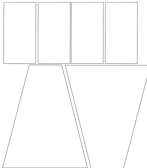
These are the 3D drawings which were then laser cut on acrylic sheets. The wind tunnel was constructed from the laser-cut acrylic sheets, which were then assembled using hot glue and tape to ensure a sturdy and airtight structure.
