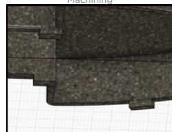
Figure 8.11: 2mm Machining Standoffs
