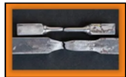
Figure 1.8: Final Break After Elongation Test Credit: hzo.org
