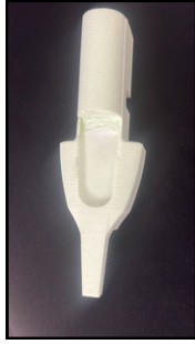
Fig 9.1: Rejected Car Body with machining Issues
