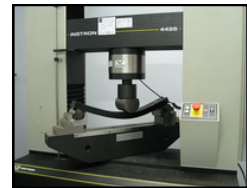
Figure 7.6: Universal Testing Machine Credit: Wikipedia
